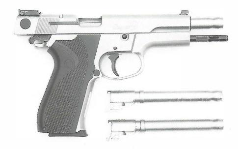
The complete package includes a gun and three runs, respectively in 9 mm Para, 9x21 and .356 TSW. The constriction near the mouth is necessary to get the walk out of the tightly fitting bus.
